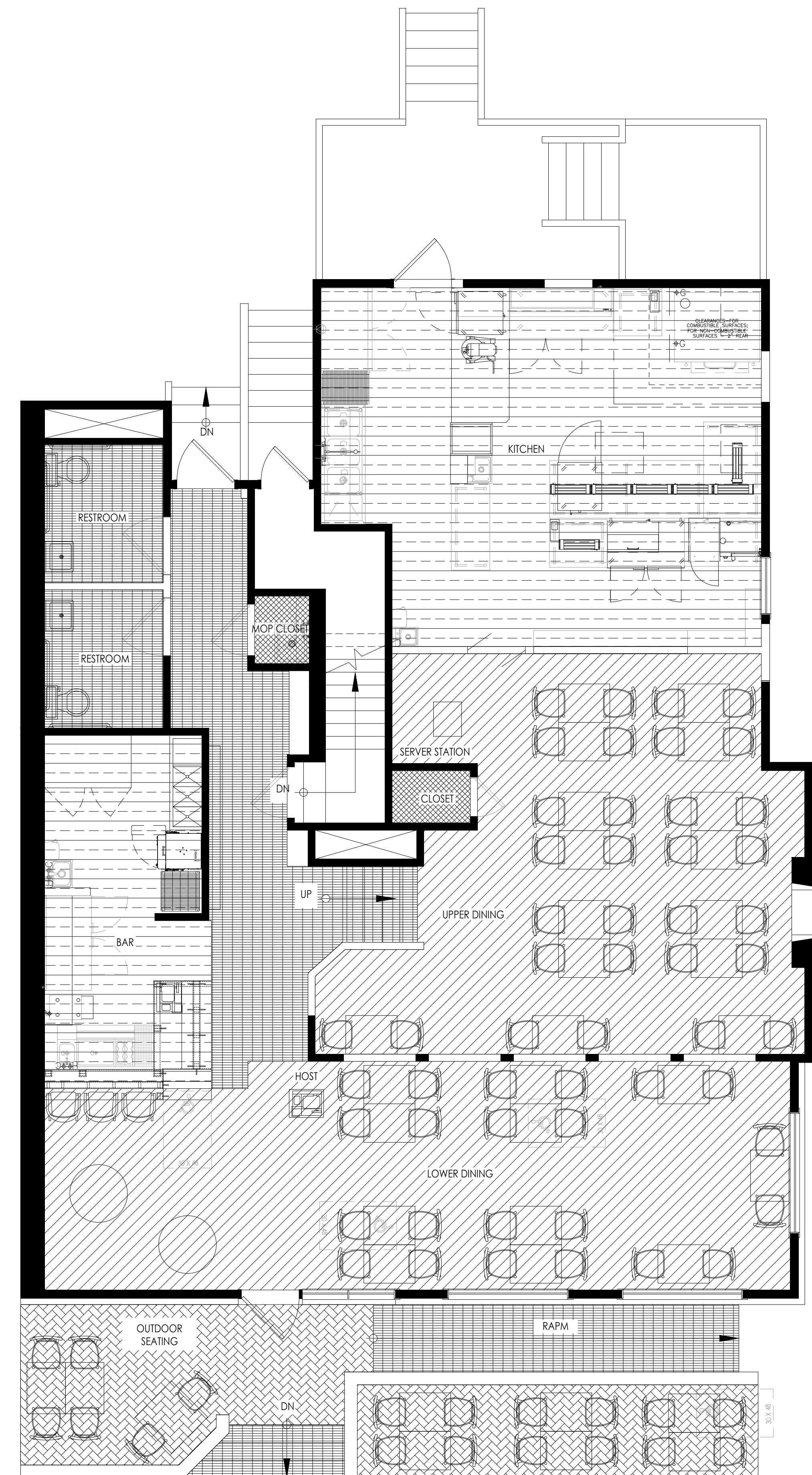
2 FIRST FLOOR - OCCUPANCY FLOOR PLAN 1/4" = 1'-0"
